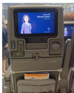
➊ Economy class features an 11.1in touchscreen IFE monitor that removes the need for a separate handset. Note the rectangular NFC reader on the left side just above the table. ANDREW WEST/SIA
